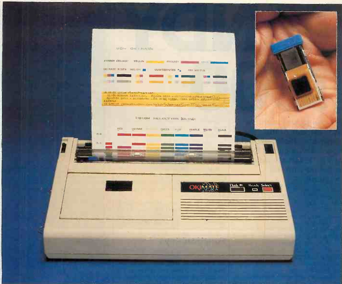
Above: The Okimate produces exceptionally bright and clear colours. Top right: The colour ribbon is divided into sections of yellow, magenta and cyan. Below: The thermal print head contains 24 heating elements which melt the dye on to the paper.
